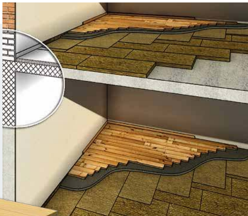
Sound insulation of floating floor with FIBRANgeo B-571
