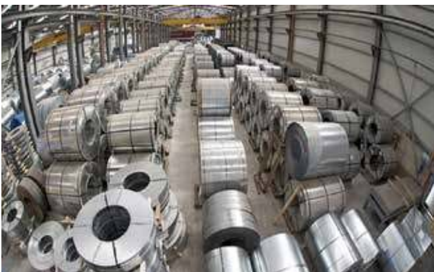
Galvanized steel coils cut to size for FIBRANprofiles production
